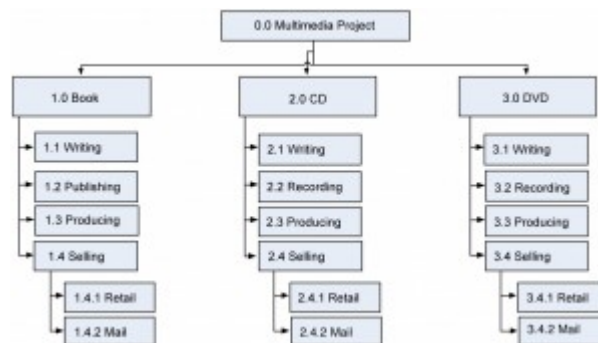
Figure 9.5: A WBS for a multimedia project Source: Project Management Skills for All Careers
